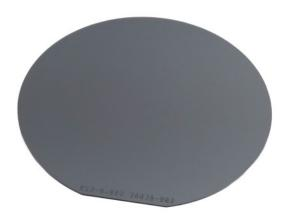
RESISTANCE NEED NOT BE FUTILE. Resistivity Standards (RS) span 4 decades and are designed for calibrating both contact and non-contact resistivity measuring instruments. The standard contact resistivity measuring instruments. The standard is created by sawing a doped single crystalline ingot into wafers, lapping and chemically cleaning them to VLSI Standards' specifications.
