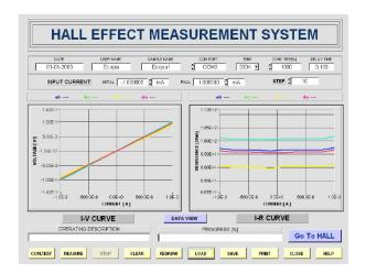
Soft calcul automatically all the electrical parameters of your sample and display the result. It is also possible to check the ohmic contact by trace I(V) curve
