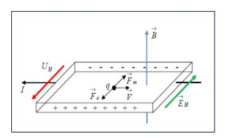
Hall effect Measurement Systems allow the ultra-fast characterization of several intrinsic parameters of conductive, semi-conductive materials. They use the Van Der Pauw method which is perfectly suited to thin film measurements and the Lorentz force in order to monitor around ten characteristics simultaneously under different environmental constraints.
