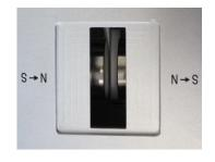
By moving the pull-out-shelf, the gap between the two magnet is adjusted.
