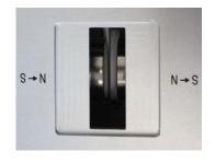
By moving the pull-out-shelf, the gap between the two magnet is adjusted.
