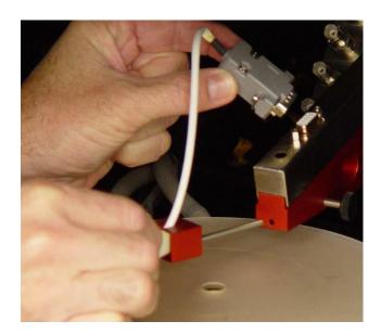
Photo: L-4PQM quick mounting block, holding SP4-62085TRQ mounted to our QuadProII S-A8 resistivity test station
