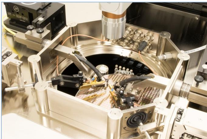
Sample Probe Configured with 2 RF + 2 COAX Probes
