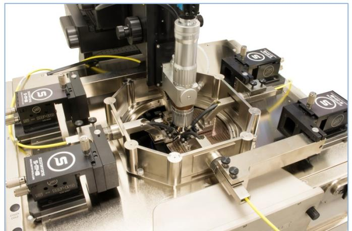
Sample Probe Configured with 4 RF Probes
