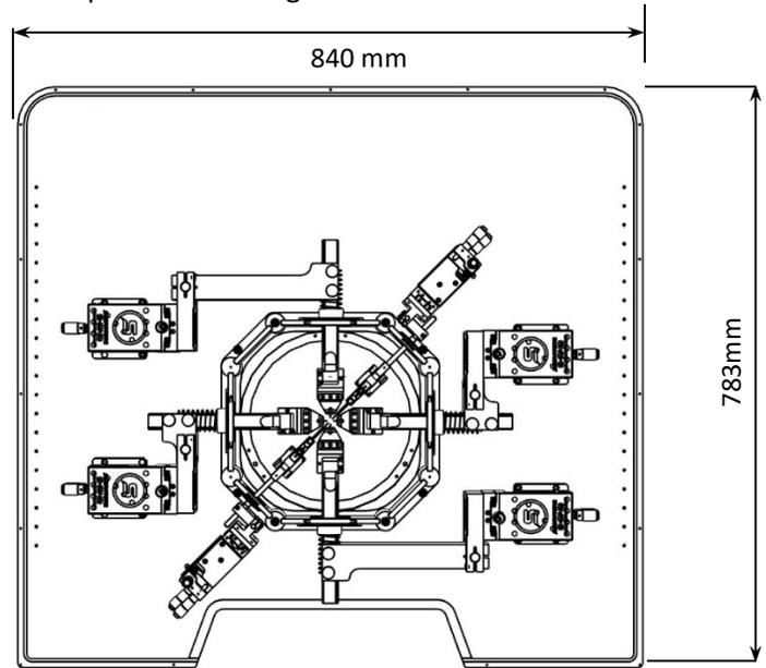
Sample Probe Configured with 4 RF + 2 DC Probes
